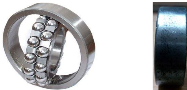
Figure 2 Healthy Bearing 2205 And Faulty Bearing 2205
